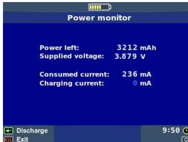
Figure 4.5: „Power monitor” working state
